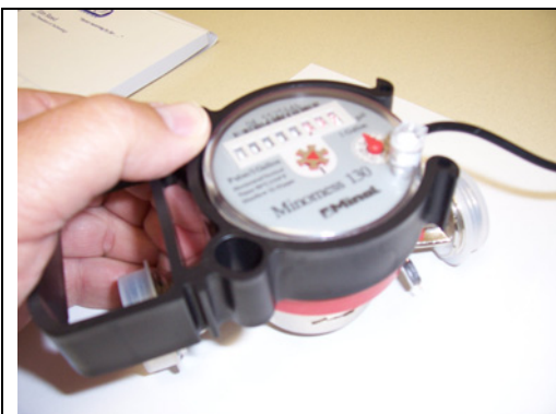
Illustration 5.10.6 C Shows the Meter Clamp placed around the meter register.
